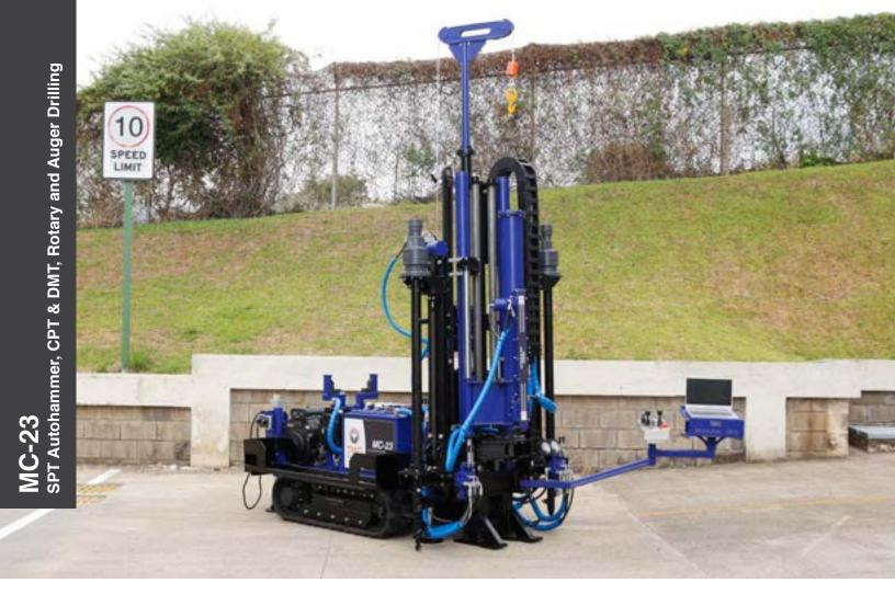
The MC-23 is a small, yet powerful multipurpose geotechnical drill rig. With a built in SPT autohammer, a powerful rotary auger drill head, dual anchor masts and 20 ton twin hydraulic drive cylinders that allows for 20 ton CPT testing, DMT testing, Shelby tube testing and direct push sampling, the MC-23 is the smallest and most powerful multi-function rig on the market.
