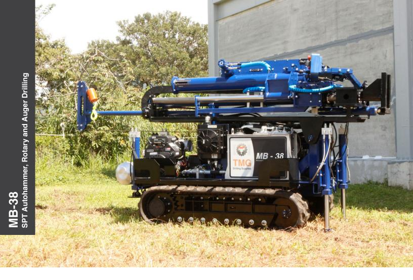
The MB-38 is a small, portable, and easy to use rotary drill rig with an SPT autohammer soil sampling system, which can be mounted on a small truck, on trailer or on rubber tracks.
