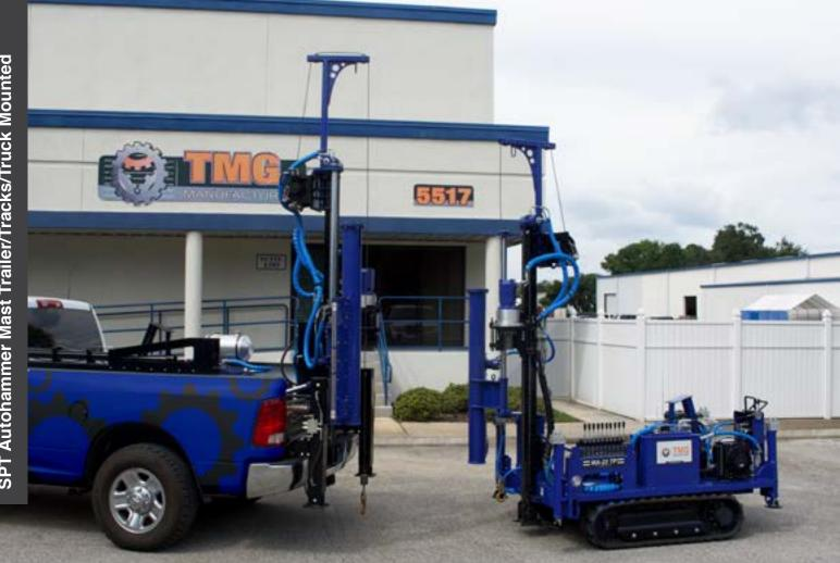
The MA-23 is a small, portable, and easy to use rotary drill rig with an SPT autohammer soil sampling system, which can be mounted on a small truck, on trailer or on rubber tracks.
